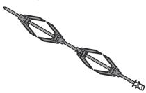
Once you have prepared the rotisserie rod, place it on the supports. Insert the tip of the rod in the housing of the mechanism on the left-hand support until it stops.
