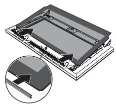
5. Remove the intermediate glass pane by lifting it upwards.
