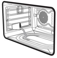
• Spray a water and washing up liquid solution inside the oven using a spray nozzle. Direct the spray against the side walls, upwards, downwards and towards the deflector.
