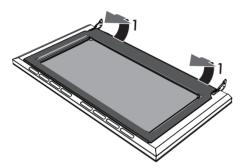
4. Pull the internal glazing pane from the front strip (2) to remove it from the door.
