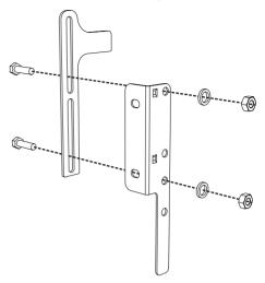
4. Align the base of the hook on the fastening bracket with the base of the slot on the wall fastening plate.
