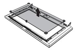
6. Clean the external glass pane and the panes removed previously. Use absorbent kitchen roll. In case of stubborn dirt, wash with a damp sponge and neutral detergent.
