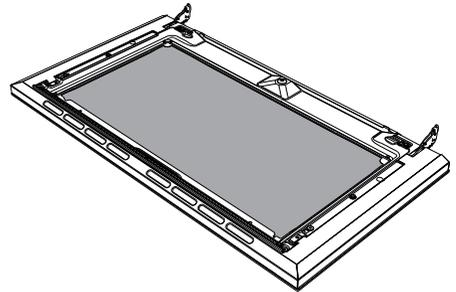
7. When you have finished cleaning, reinsert the intermediate glass pane in its housing in the door.
