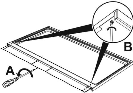
2. Place the upstand on the hob. Align the 6 bottom slots of the upstand with the 6 screws on the back of the hob that were previously loosened.
