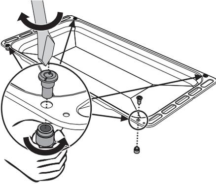
2. Position the rotisserie supports in the bushings as shown in the figure below.
