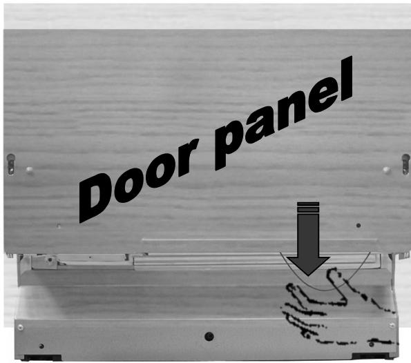
An "emergency" hand-operated system allows the dishwasher to be opened in the event of a power outage. This consists of a string (accessible from the bottom at the front, even with the door mounted) which releases the door when pulled down.
