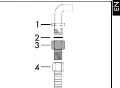
Carefully screw the hose connector 3 to the appliance's gas connector 1 (1/2" thread ISO 228-1), placing the seal 2, provided, between them. Apply insulating material to the thread of connector 3 and then screw the steel hose 4 onto the connector 3.
