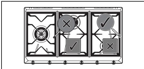
When cooking, to avoid burns, damage to the hob or top, all containers or steak pans must be positioned within the perimeter of the hob.
