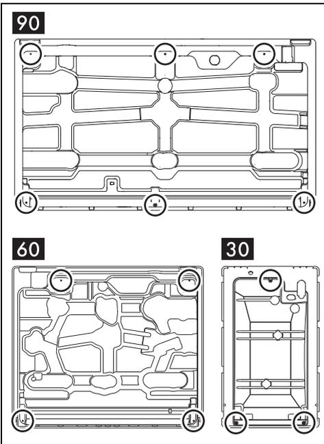
Screw the fixing brackets into the dedicated holes as shown to properly fasten the hob to the built-in structure.
