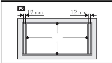
2. Use light pressure to make the seal stick to the edge around the hole cut in the worktop.
