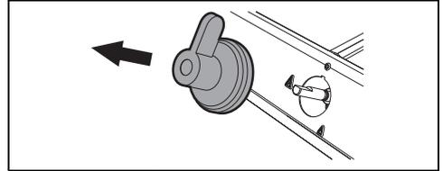
3. Remove the flame-spreader crowns and relative burner caps.
