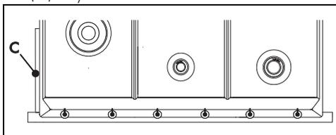
**!** Do not use silicone to secure the hob. This would make it impossible to remove the hob without damaging it.
