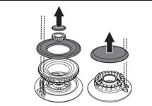
Before lighting the hob burners, make sure that the flame-spreader crowns are correctly positioned in their housings with their respective burner caps. Make sure that the holes in the burners are aligned with the igniters and thermocouples. Also ensure that the flame-
