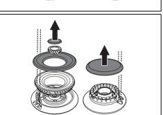
Before lighting the hob burners, make sure that the flame-spreader crowns are correctly positioned in their housings with their respective burner caps. Make sure that the holes in the burners are aligned with the igniters and thermocouples. Also ensure that the flame-spreader crowns are correctly engaged in the burner holes
