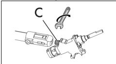
8. Use a spanner to remove the nozzles "C" and install the new ones for the required gas supply, following the indications given in the
