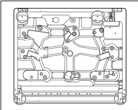
Screw the fixing brackets into the dedicated holes as shown to properly fasten the hob to the built-in structure.
