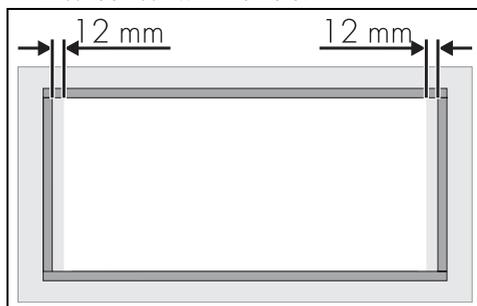
2. Use light pressure to make the seal stick to the edge around the hole cut in the worktop.
