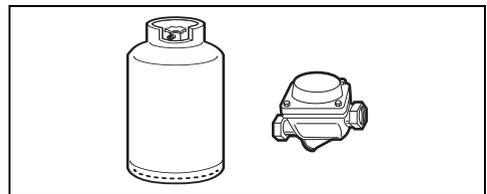
Use a pressure regulator and make the connection on the gas cylinder following the guidelines set out in the standards in force. The supply pressure must comply with the values indicated in the "Burner and nozzle characteristics table".
