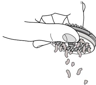
The multi-food grinder accessory body, feed screw, fastening ring nut, cutter and the three grinder discs must not be washed in a dishwasher. They should be washed by hand using lukewarm water and neutral soap.
