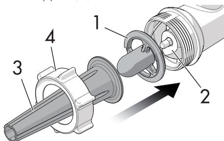
3. Insert the fastening ring nut (4) and screw it onto the body of the multi-food grinder, without overtightening.
