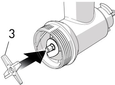
2. Position one of the three grinder discs (4) supplied on the cutter (3), according to the final texture you wish to obtain.
