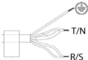
For 380-415V 3N or 380-415V 2N, separate with the scissors the wires as showed in the image below and connect them.
