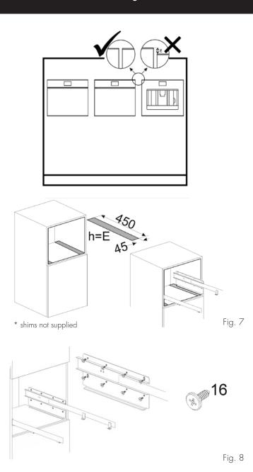
Fasten the brackets using all the necessary screws.
