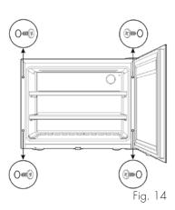
7. Adjust the hinges of the doors around the products in order to make the gaps uniform.
