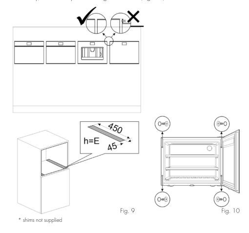
5. Adjust the hinges of the doors around the products in order to make the gaps uniform.
