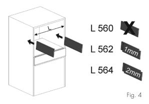
Place the runners on the shelf of the unit whilst keeping them flush with the side of the unit.
