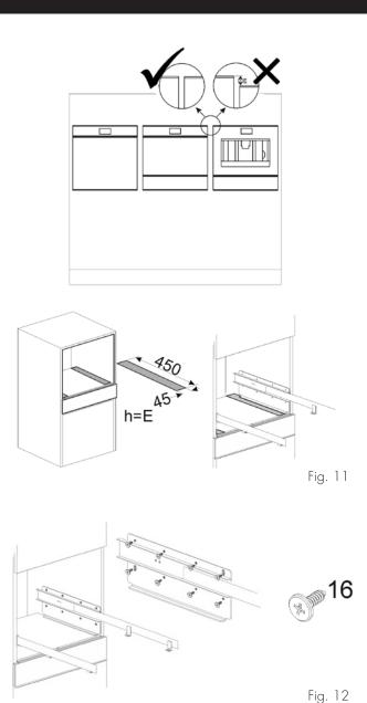
Fasten the brackets using all the necessary screws.
