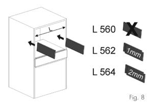
Place the runners on the casing of the drawer whilst keeping them flush with the side of the unit.
