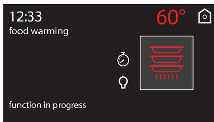
6. While the function is in progress, it is possible to set a timer for a maximum of 4 hours (see "Timer during function"), a warming duration (see "Timed cooking") or a delayed warming (see "Delay cooking"). Press the
