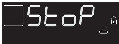
3. The door remains locked until the temperature inside the oven returns to a safe level. Wait for the oven to cool down (the indicator light
