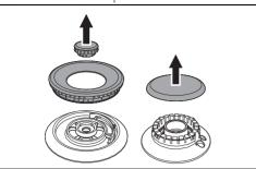
Remove the gasket on each burner's thermocouple and igniter.
