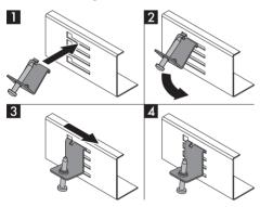
Place the hob on the insulating seal and fix it to the supporting structure using the supplied screws and fastening brackets (A) so that the hob is perfectly level.
