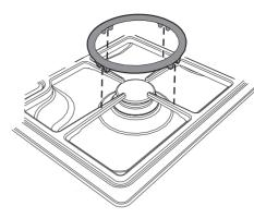
The ring must be placed under the hob grid as shown in the picture above.
