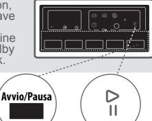
To avoid programme flow from being affected if programme buttons are pressed or programme button is turned when performing washing operation in your machine, child lock is available.
