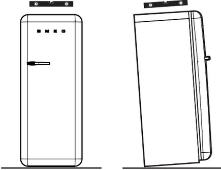
A few days after installation, check that the initial level adjustment is still correct. Make sure that the appliance is still stable and the door seals still close hermetically when it is in operation and loaded with food. If necessary, re-adjust the level and the seals.
